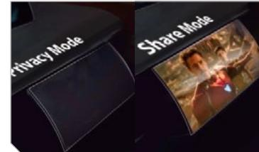
**Passenger's Viewing Angle Control Display**
